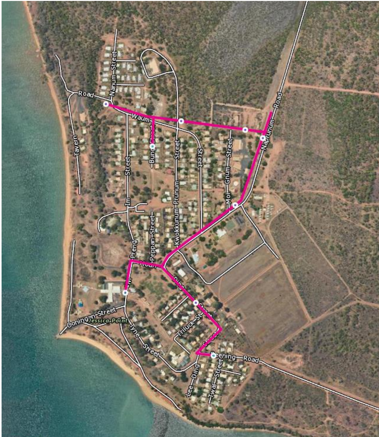
Figure 14: Napranum 11kV distribution network
