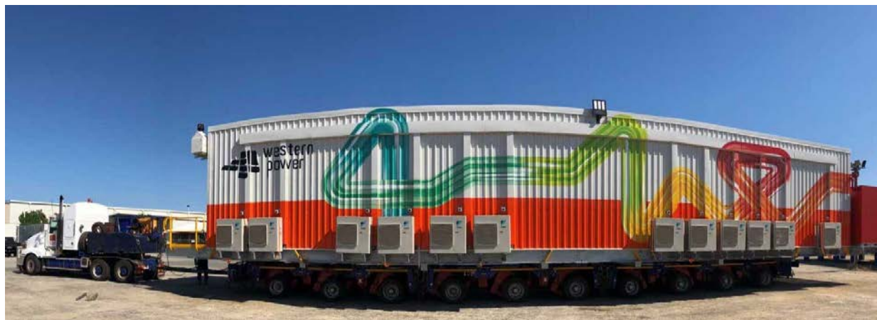
Figure 49 Kalbarri battery being transported from Perth 126
