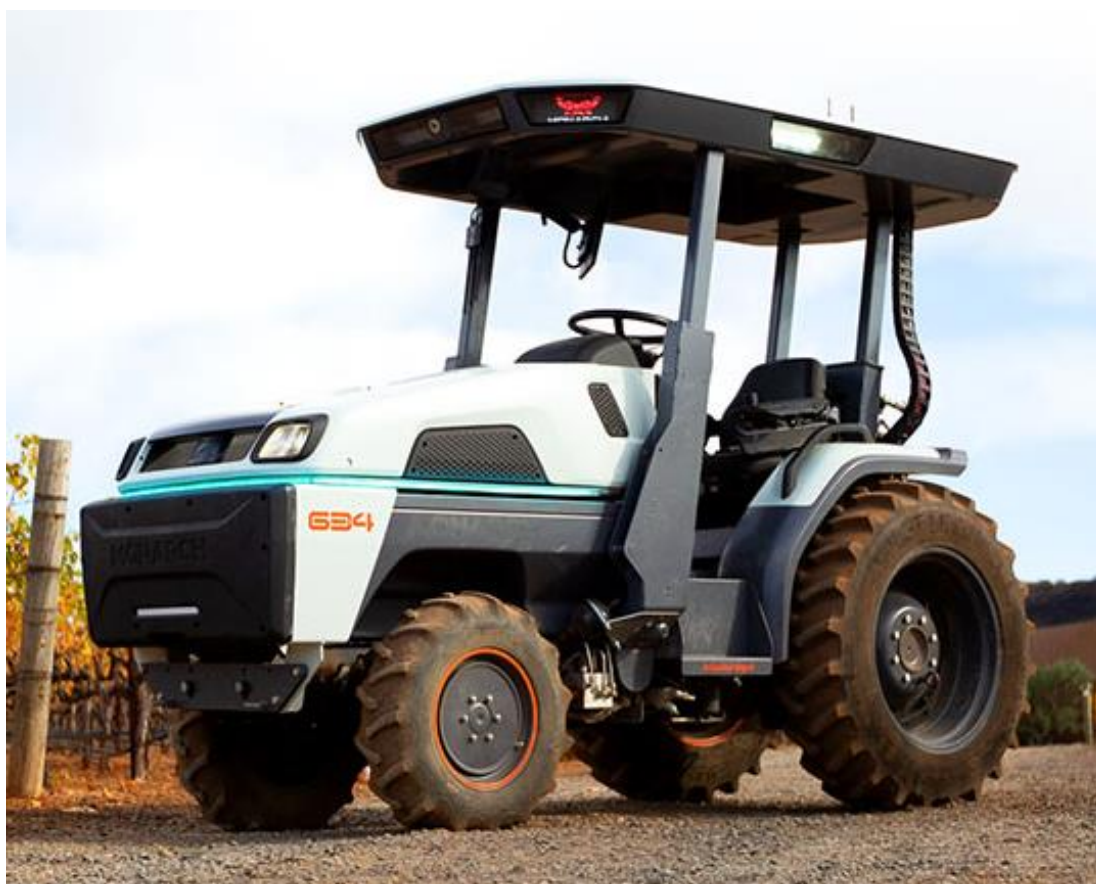
Figure 31 Monarch electric tractor that can operate autonomously without a driver 70
